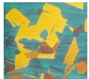
Figure 2. Increasing the Nickel Content Changes the Microstructure of a Stainless Steel from Ferritic (left) to Duplex (middle) to Austenitic (right) (These pictures, courtesy of AvestaPolarit, show polished and etched samples, enlarged under a light microscope. In the duplex structure, the ferrite has been stained so that it appears as the darker phase.)
