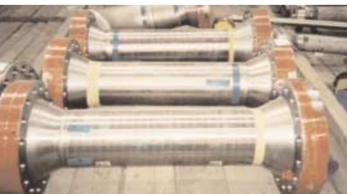
2205 Spool Pieces (Source: Arco Exploration and Production Technology)
