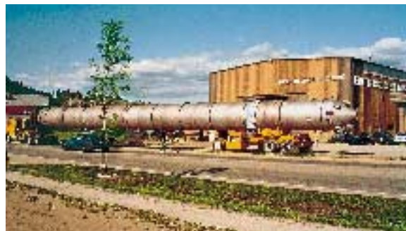
2205 Oxygen Delignification Reactor, Enterprise Steel Fab, Kalowna, Prince George, British Columbia, Canada (Source: AvestaPolarit)
