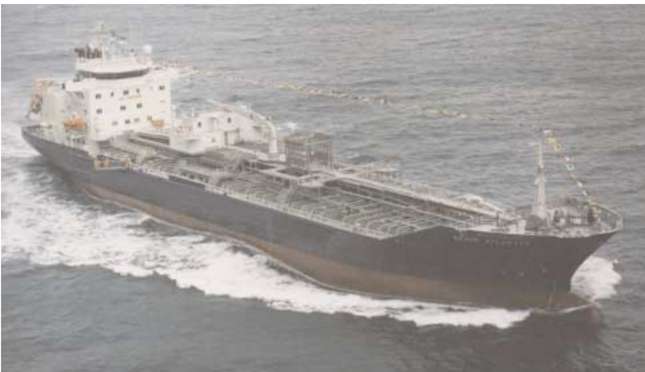
Marine Chemical Tanker with 2205 Tanks (Source: Krupp, Thyssen Nirosta)
