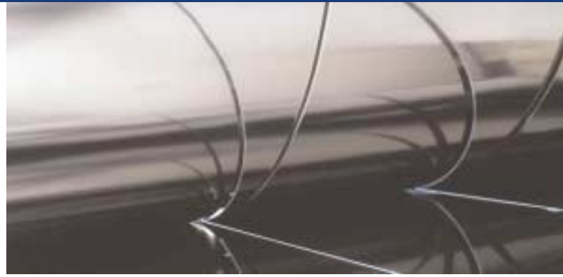
Slitting of Duplex Stainless Steel (Source: Krupp Thyssen Nirosta)
